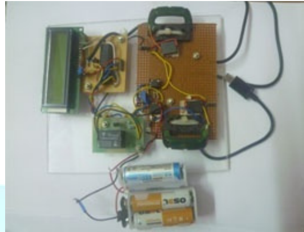
Fig. 5. RF Power harvesting system
